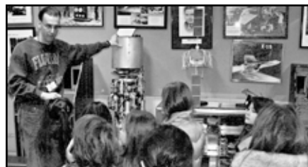
This engine, built by Reaction Motors, NJ, was used on the X-1 -- the world's first supersonic airplane.
