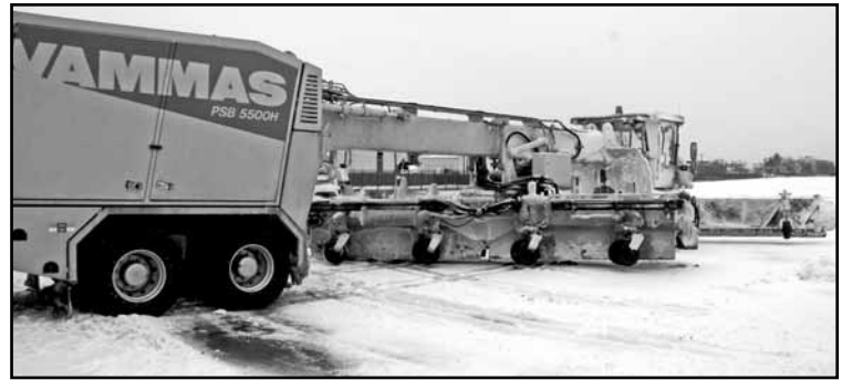
The 68' 7" long multi-functional vehicles clear the runways. Top photo rear view (l-r): snow blower, 46" diameter rotating broom that is 22' wide, operator's compartment and 30' front plow. Photo below is front view.
