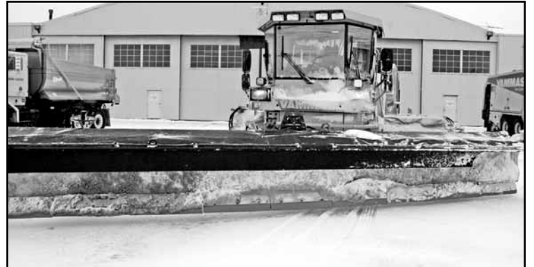
The 68' 7" long multi-functional vehicles clear the runways. Top photo rear view (l-r): snow blower, 46" diameter rotating broom that is 22' wide, operator's compartment and 30' front plow. Photo below is front view.
