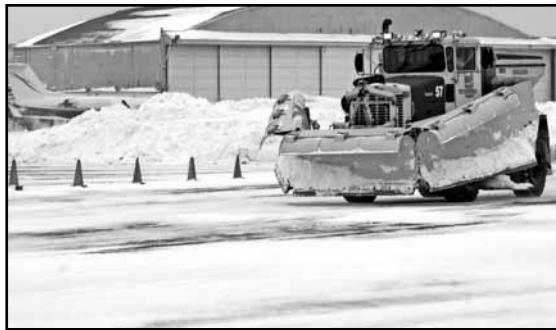
Above left is plow front view with 24' blade. Special poly blade edges safely remove snow but do not damage in pavement navigational lights. Above right is truck with plow folded for transport.
