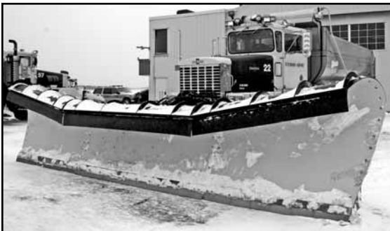
Above left is plow front view with 24' blade. Special poly blade edges safely remove snow but do not damage in pavement navigational lights. Above right is truck with plow folded for transport.
