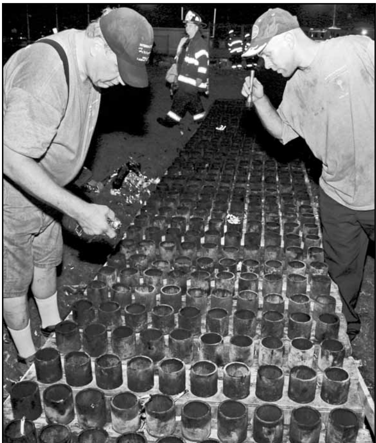
After the show, each firing tube was inspected for unspent rounds. Suspect tubes with rounds were identified, and would be removed safely back at the contractor's operation.
