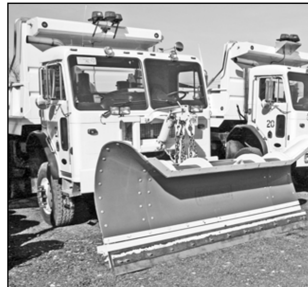
Special poly blades are used on the snow plow.
