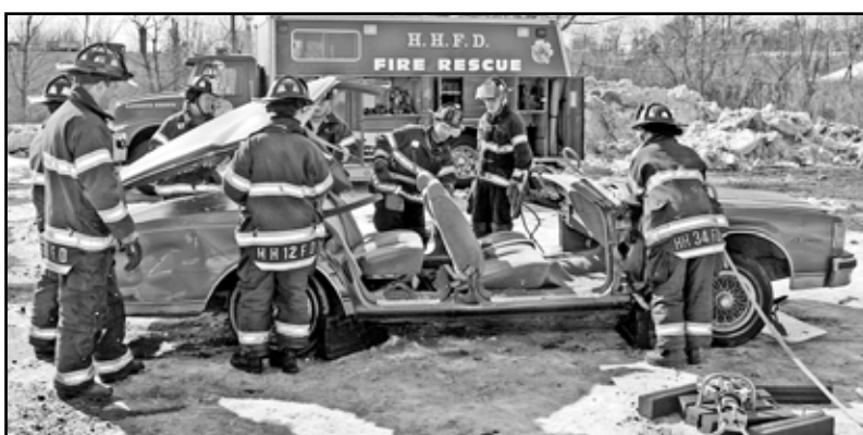
Removing the roof away from the vehicle.
