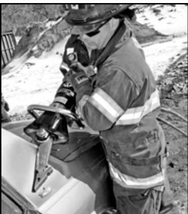
Cutting off the rear roof support. Gas cylinders may be hidden in this support.
