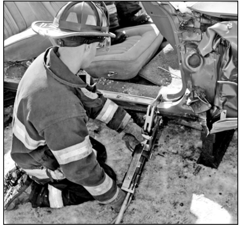
Extra care is needed in cutting the frame. Air bag gas cylinders or hybrid high voltage cables may be hidden here.
