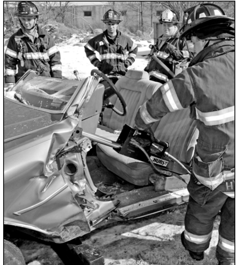
Once the frame has been cut, the front section of the car is spread open by the ram tool to extricate patients.
