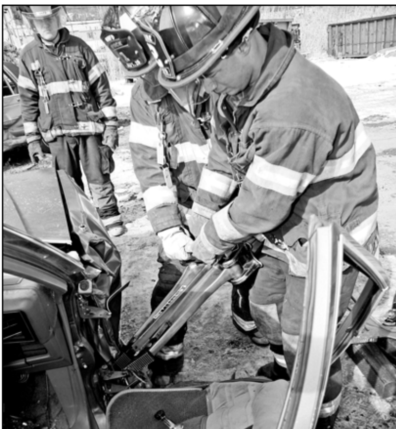
"Jaws of Life" spreader tool detaches passenger side door.
