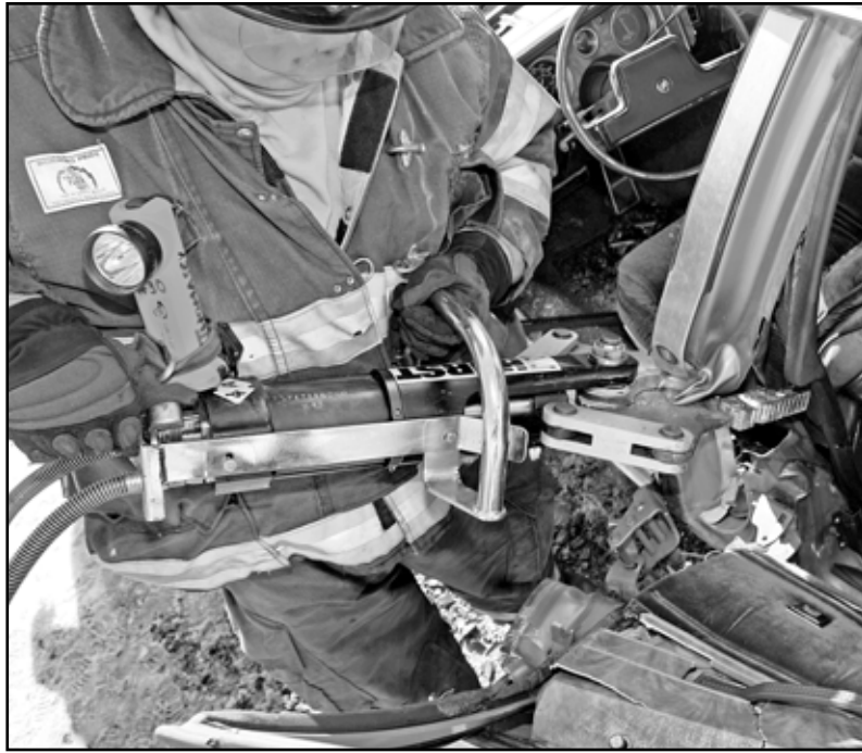
Cutting the center post and creating the third door. Air bag gas cylinders may be hidden in this post.
