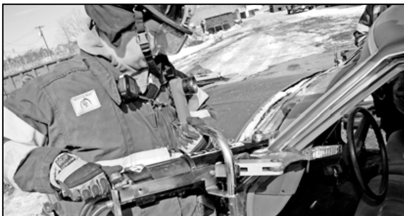
Cutting off the roof front support, after the glass has been removed. Air bag gas cylinders may be hidden in this support.
