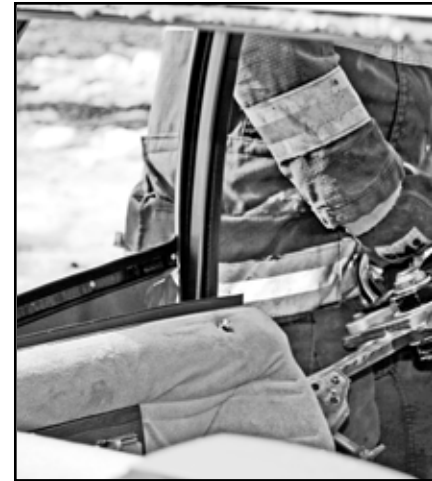
View of door being spread open from inside.
