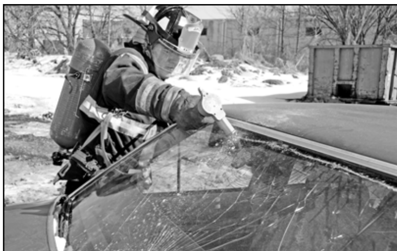
Cutting the laminated front windshield using an air tool.
