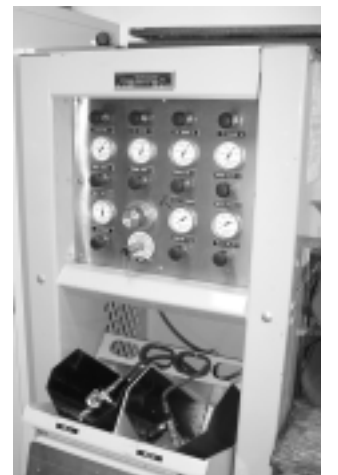
Unit that is used to refill air tanks.
