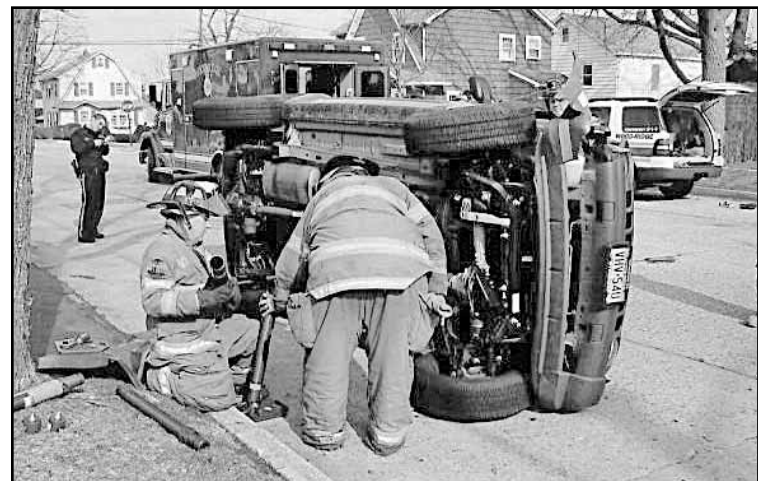
Wood-Ridge firefighters preparing to stabilize the vehicle using the Paratech System.
