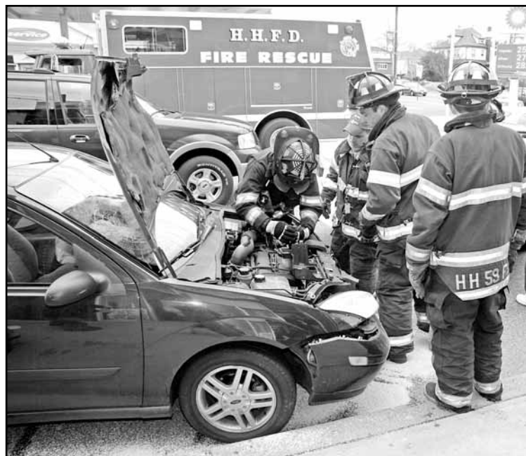
The Department applied Speedy Dry to absorb leaking fluids, pried open the hood and disconnected the battery of the last vehicle.
